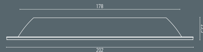
DM 512 ED: 202 cm ID: 178 cm D: 23,5 cm Fibre Reinforced Plastic (FRP)
